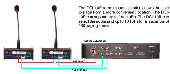
Please note that two connections are required between the 10R and 10P. The remote link cable is a standard RJ-45 type commonly used for computer networks. The cable supplied with the unit is for test purposes only. The audio cable required is standard shielded-type 1/4" phone plugs. The length can be up to 200 meters.
